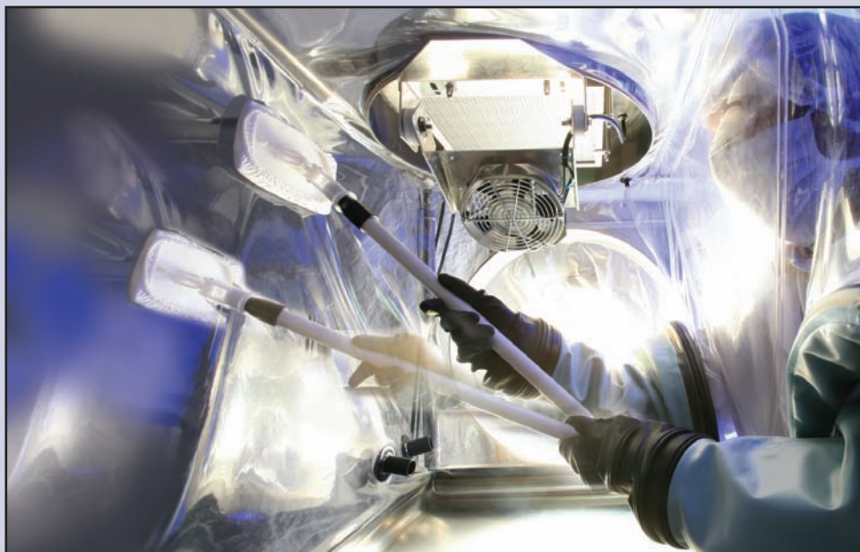
Fig. 1 - Wipe surfaces using parallel, overlapping strokes
