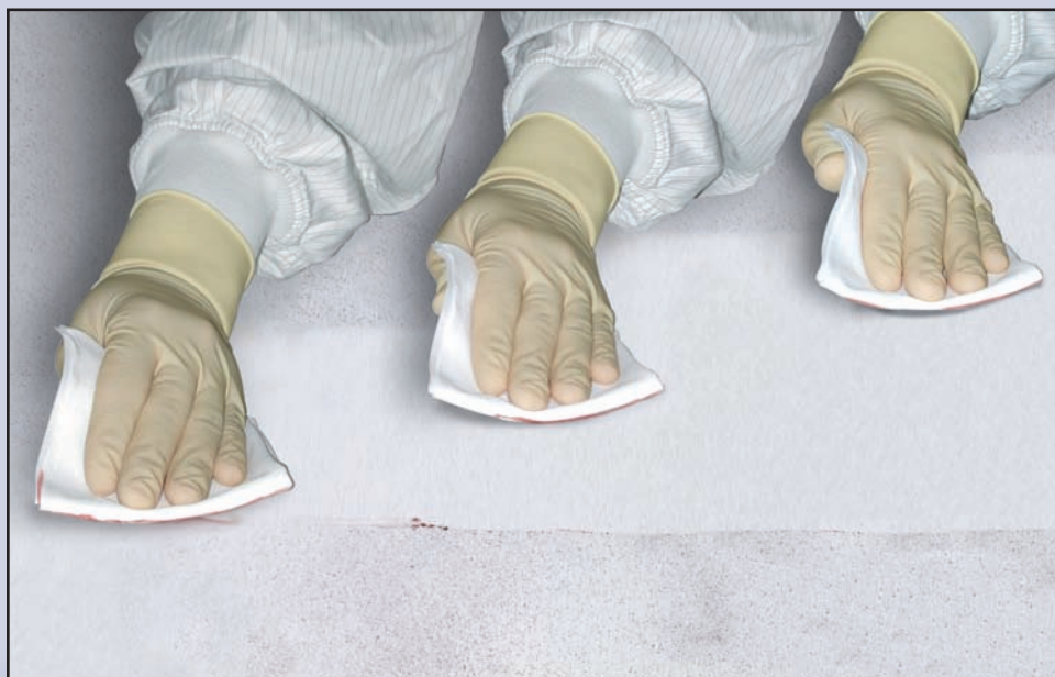
Fig. 2 - Wipe surfaces using parallel, overlapping strokes
